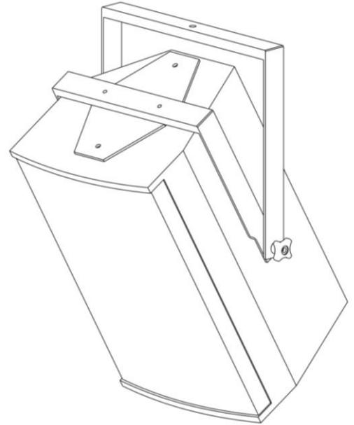
Ensure that an M8 eyebolt is secured to the rear point on the EMS-122 enclosure to use as a secondary safety.
