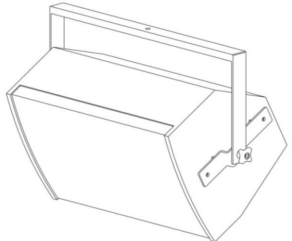
Ensure that an M8 eyebolt is secured to the rear point on the EMS-122 enclosure to use as a secondary safety.
